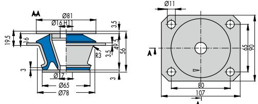
Fig. 22 Conical Mount 057 18 804
