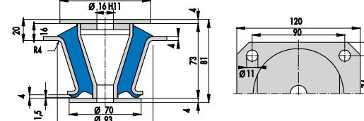
Fig. 24 Conical Mount 057 18 806
