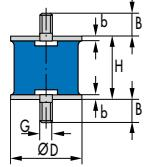
Fig. 6 Circular Mounts Type A, constricted-body elastomer contour
