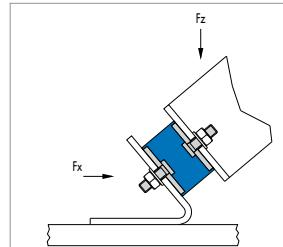
Fig. 3 Compressive and shear loading
