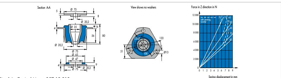
Fig. 14 Conical Mount 057 18 013
