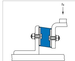
Fig. 5 Shear loading
