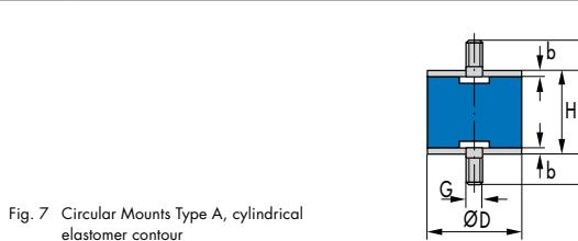
Fig. 7 Circular Mounts Type A, cylindrical elastomer contour
