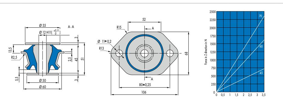
Fig. 26 Conical Mount 057 18 816
