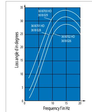
Fig. 5 Transient of the loss angle as a function of frequency
