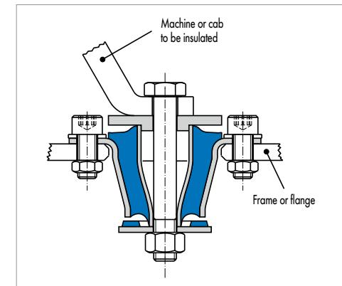
Fig. 4 Secured by threaded fasteners in flange
