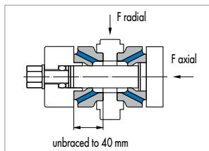
Fig. 2 Fitting & installation instructions:
