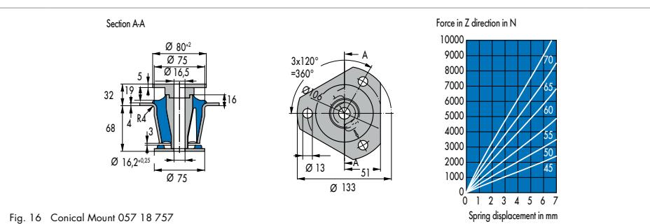
Fig. 16 Conical Mount 057 18 757
