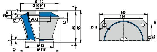
Fig. 25 Conical Mount 057 18 807
