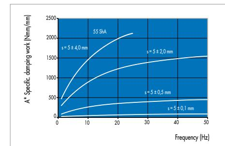
Fig. 5 Specific damping work, 036 18 704; 55 ShA
