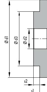
Fig. 3 Type II Centering Washer, single-tier
