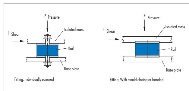
Fig. 3 Fitting &amp; installation: rails with load directions
