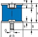
Fig. 10 Circular Mounts Type B, constricted-body elastomer contour
