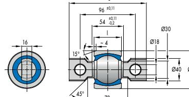
Fig. 5 Spherical Mount 054 18 710, 054 18 711
