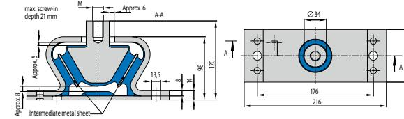
Fig. 3 Tapered Mounts 033 18 720, 033 18 730
