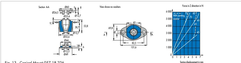
Fig. 13 Conical Mount 057 18 226
