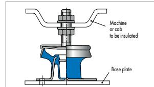
Fig. 7 Fitting &amp; installation instructions: Hydro Mount DL
