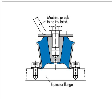
Fig. 3 Secured by threaded fasteners in base
