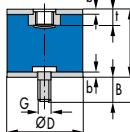
Fig. 11 Circular Mounts Type B, cylindrical elastomer contour
