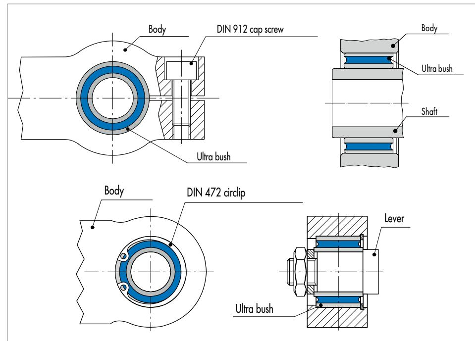
Fig. 6 Fitting &amp; installation instructions: Ultra Bushes
