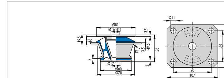
Fig. 23 Conical Mount 057 18 805
