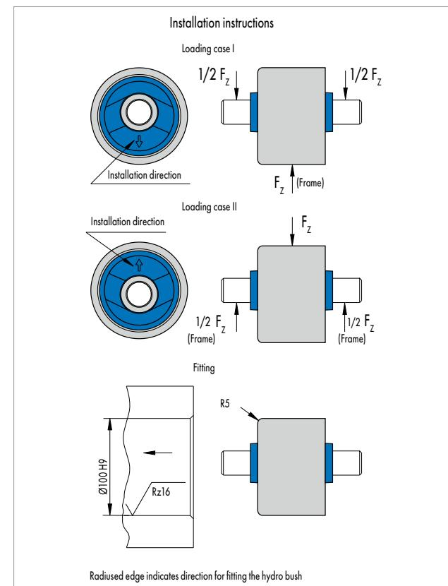
Fig. 3 Fitting &amp; installation instructions: Hydro Bushes
