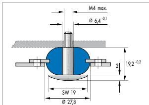
Fig. 3 Installation diagram with stud SW19
