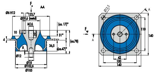
Fig. 21 Conical Mount 057 18 792
