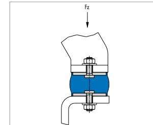
Fig. 4 Compressive loading
