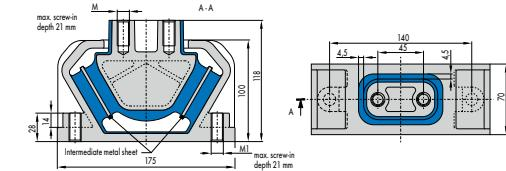
Fig. 4 Tapered Mounts 033 18 700, 033 18 701
