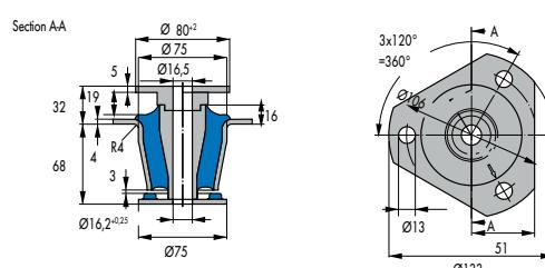
Fig. 15 Conical Mount 057 18 756
