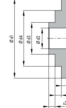
Fig. 4 Type III Centering Washer, two-tiered
