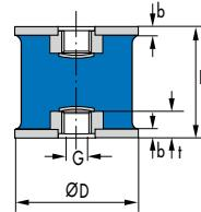
Fig. 12 Circular Mounts Type C, constricted-body elastomer contour
