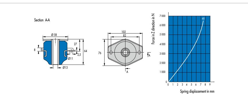
Fig. 28 Conical Mount 058 18 001
