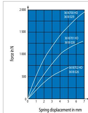
Fig. 4 Static spring characteristic curve in Z direction
