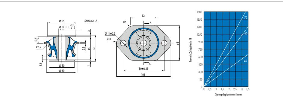
Fig. 27 Conical Mount 057 18 817
