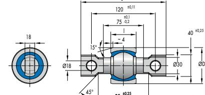
Fig. 5 Spherical Mount 054 18 732
