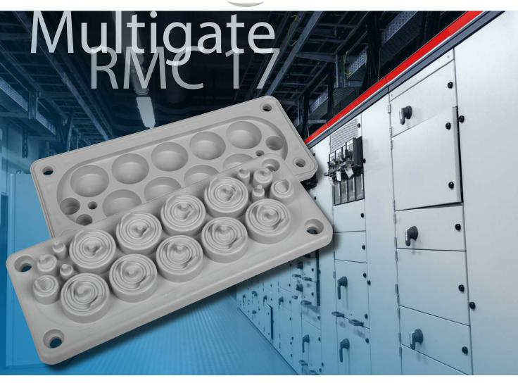
The new plastic reinforced Multigate RMC se ries takes advantage of a new patent pending sealing system. Extra sealing rings can easily be pulled off without extra tools to make RMC perfectly fit various cable sizes. Covered cable diameters for RMC 17 are from 5 to 30 mm, but RMC can also be easily adapted to custom er specific cable sizes. IP classification is IP65, and the materials are fire retarded and halogen free. RMC fits the FL21 standard cut-out.
